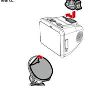
Peel off the protective plastic sheet from the adhesive bracket.
