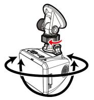
2. Then tighten the knob to make sure the camcorder is securely locked in place.
